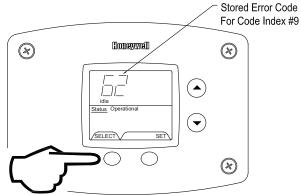
Step 6: Continue pressing the "Temperature Down" button to change to the next error code index and press "Select" to view the error code number, if any, for that index number. Continue on to index #1, the oldest error code index. The water heater display will store up to 10 error codes with the oldest code starting in code index #1 with the most recent code in code index #10.
